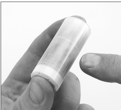
1.22 Inspect ceramic plungers for cracks and scoring to the surface. Clean with a wire-wheel brush if necessary.
