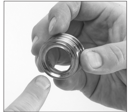
1.11 Inspect the grooved V-packing surface of the seal cases for scoring or damage.
