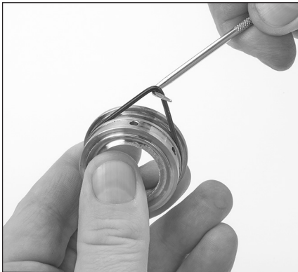
1.09 Using a pick, remove the seal case O-rings.
