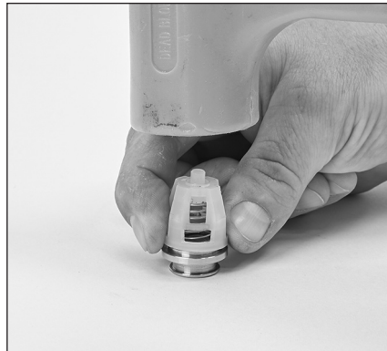
2.17 Using a rubber mallet, lightly tap spring retainers into place.
