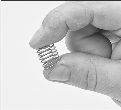
2.08 Inspect springs for proper tension or any damage.
