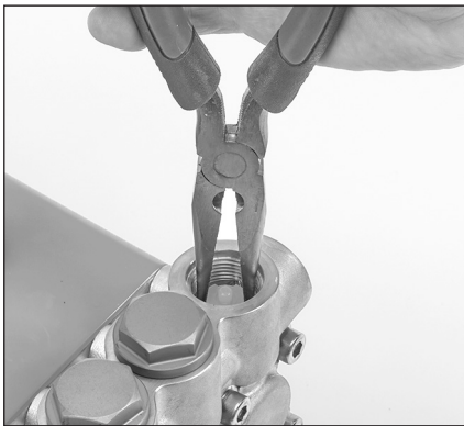
2.04 Use needle-nosed pliers to grasp the top of the spring retainers. Twist while pulling away from manifold to remove valve assemblies.
