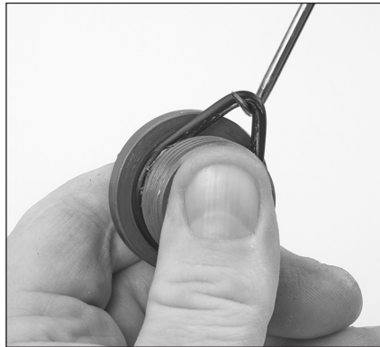
2.02 Using a pick, remove O-rings from valve plugs.
