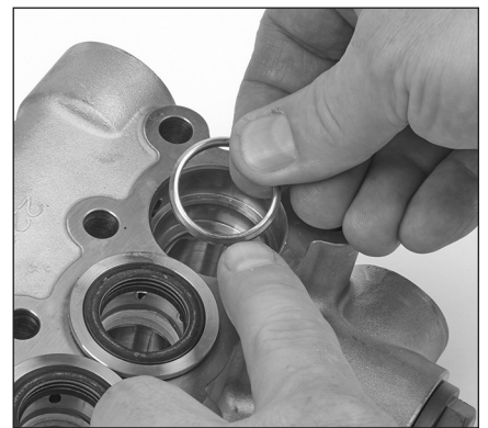
1.14 Remove the male adapters and inspect for wear or damage.
