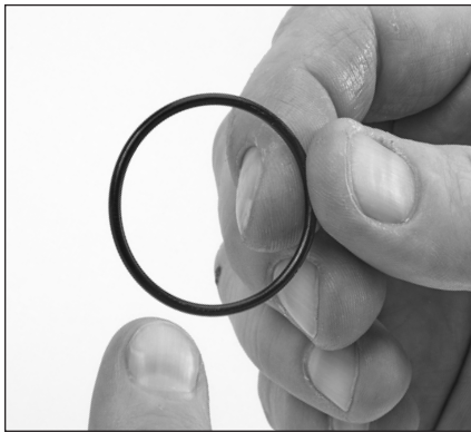
1.10 Inspect the seal case O-rings for cuts, nicks or damage.
