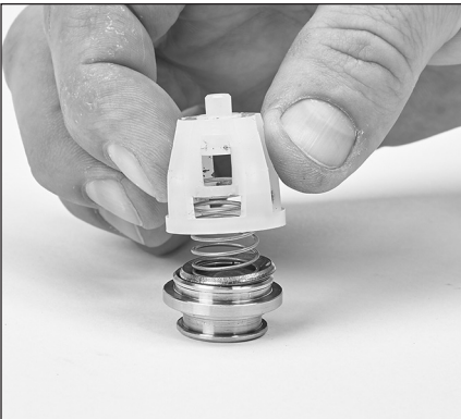
2.16 Place spring retainers onto valve seats.
