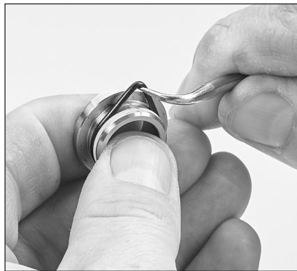
2.11 Using a pick, remove O-rings and backup rings from valve seats.
