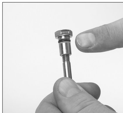
1.20 Remove the plunger retainers from the plungers and inspect the O-rings and backup rings for damage.
