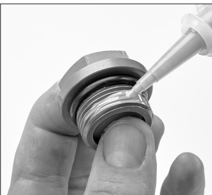
2.22 Place a few drops of Loctite® 242® on the threads of valve plugs, enough to lightly cover at least the first two threads.
