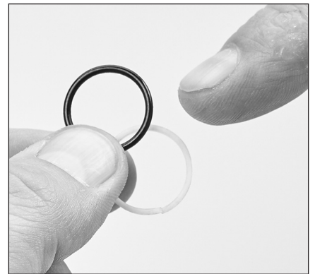
2.12 Inspect valve seat O-rings and backup rings for cuts, nicks, or damage.
