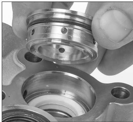
1.36 One side of the seal cases have a groove. Install grooved sides facing down into the manifold and press them into place.
