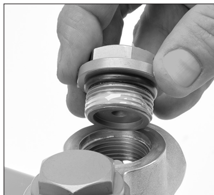
2.23 Install valve plugs into manifold and thread by hand.
