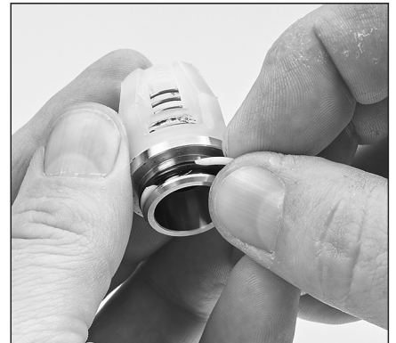
2.18 Replace valve seat O-rings into the top of the groove, then backup rings at the bottom.
