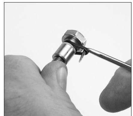
1.21 Using a pick, remove the plunger retainer O-rings from the plunger retainers.
