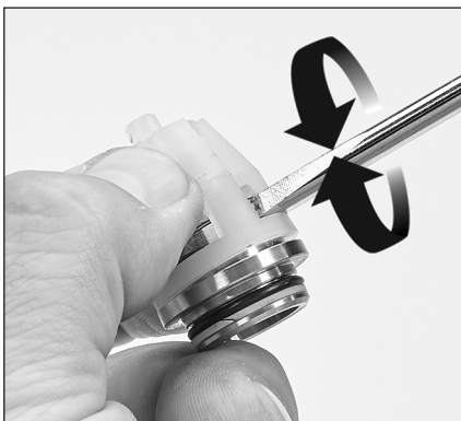
2.05 Insert a flat tip screwdriver through spring retainer just above valve. Twist to create a small gap between valve retainers and valve seats.
