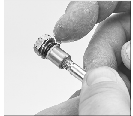
1.26 Apply a lubricant to outside surfaces of the plunger retainer O-rings.
