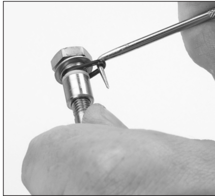
1.25 Install new plunger retainer O-rings between backup ring and head of the retainer.
