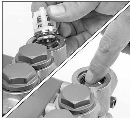
2.20 Insert valve assemblies into manifold and press into place.
