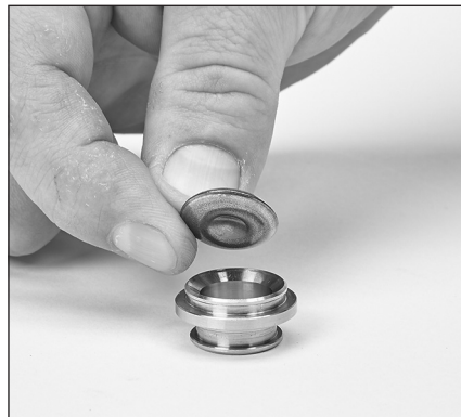
2.14 Place valves onto valve seats with tapered surfaces facing down.
