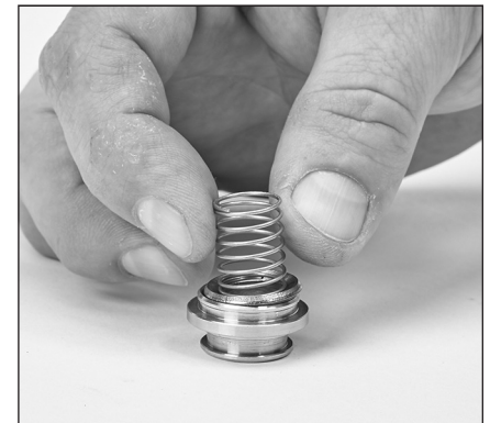
2.15 Place spring onto concave sides of valves.
