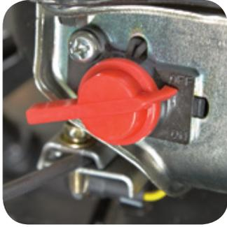
1. Turn engine/motor to Off position.
