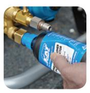
Squeeze bottle to inject pump protector fluid into pump.
