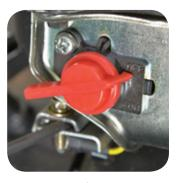
1. Turn engine/motor to Off position.
