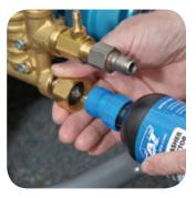
6. Screw bottle into garden hose fitting on inlet of pump.
